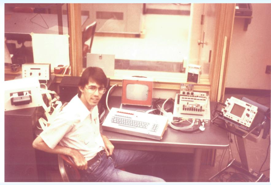
My personal hobby computer 8-bit 6502 Microprocessor 4 MHz 4K Bytes of main memory Hand "wire-wrapped" Paper tape reader Hand wound transformer on power supply. Note – base of SYMBOL computer
