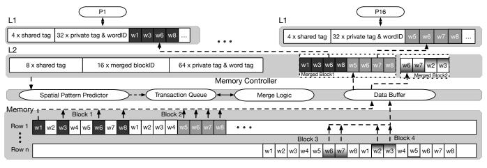
Fig. 1. The proposed design with 16 private 4-way L1s and a shared 8-way L2 cache.
