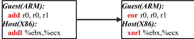
Fig. 3. An example of generalizing the opcode.
