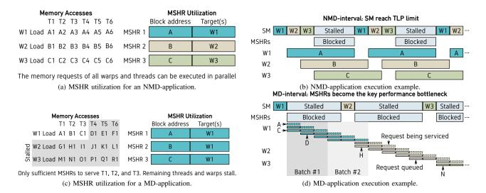
Fig. 4: Example explaining why MSHR utilization results in significantly different performance-related behavior for NMD and MD-applications. *MD-applications puts immense pressure on the L1 cache MSHRs and thereby severely limit the GPU's ability to use TLP to hide memory latencies.*
