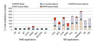
Fig. 3: L1 miss latency breakdown for selected GPU compute applications. *Delays due to insufficient MSHRs as well as queuing delays in the NoC and DRAM subsystem significantly affect the overall memory access latency of MD-applications, while NMD-applications are hardly affected.*
