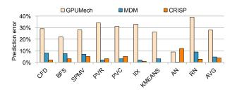
Fig. 13: Error when predicting the relative performance difference at 1.4 GHz versus 2 GHz for the MD-applications for GPUMech, CRISP and MDM. *The general-purpose MDM model achieves similar accuracy as the special-purpose CRISP.*
