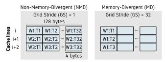
Fig. 2: Cache behavior for the example kernel in Listing 1.
