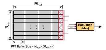
Fig. 15: Column-major partitioning of PFT to reduce PFT buffer size (4 partitions in this example). Each time the PFT buffer is filled with only one partition. Since reduction (max) is applied to each column independently, the column-major partitioning ensures that all the neighbors of a centroid are present in the PFT buffer for aggregation.
