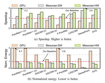
Fig. 18: Speedup and energy reduction of <u>MESORASI-SW</u> and <u>MESORASI-HW</u> over the baseline (GPU+NPU), which is twice as fast and consumes one-third of the energy compared to the GPU, indicating an optimized baseline to begin with.
