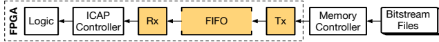
Fig. 9: Runtime partial reconfiguration engine. Augmentations to existing hardware on the Zynq board are shaded.
